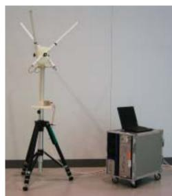
Radio field intensity measuring device with receiving antenna for measuring radio waves at mobile phone base stations
