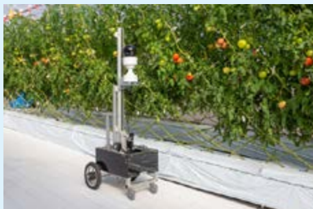
Robot equipped with a 4K camera. The remotely controlled robot moves around the greenhouse to carefully check the condition of tomatoes.
