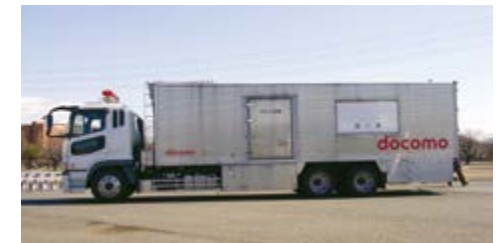
Large-scale power supply vehicle for powering communications buildings
