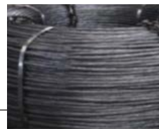
Outer armor wire properly coiled
