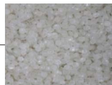
High-purity polyethylene used for outer cover can be sold at high price if completely separated and pelletized
