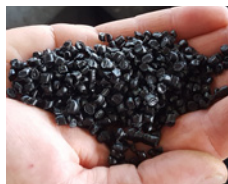
Coal tar coating for armor wire completely separated and pelletized
