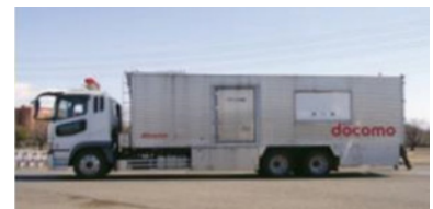
Large-scale power supply vehicle for powering communications buildings
