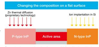
Conventional compound semiconductors are fabricated by depositing layers vertically, which makes it difficult to produce thin films. NTT developed a technology that enables composition changes on a flat surface.
